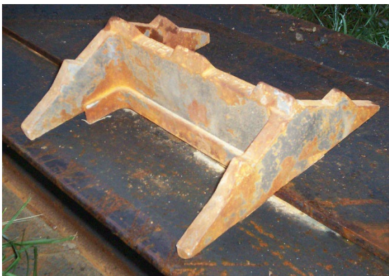
Figure 9 Bottom of H-Pile Shoe Tip
