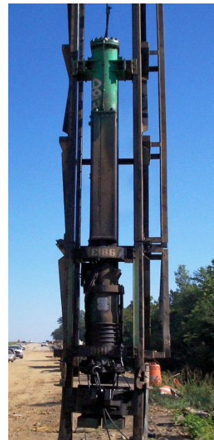
Figure 3. Photo of a Single Acting Diesel Hammer
